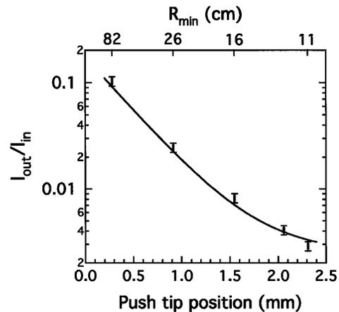
FIG. 2. Transmittance versus the push tip position and minimum radius of curvature ( $R_{\min}$ ) for Mo  $K_\alpha$  radiation on a bent 18 mm long Si mirror. Solid curve is the prediction from ray tracing calculations.
