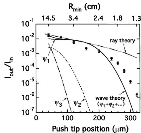
FIG. 3. Transmittance for a 5 mm long Si mirror. Dotted and solid curves are predictions from a ray tracing calculation and a simple wave-optical model, respectively. Dashed and dash-dotted curves  $\psi_1$ ,  $\psi_2$ , and  $\psi_3$  are calculated contributions from the three lowest bound states in the wave-optical model.
