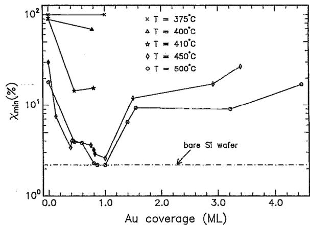
FIG. 3. Plot of  $\chi_{\min}$  vs Au coverage at several temperatures, for a deposition rate of 3 Å/s. At temperatures below 410 °C, Si films grown with or without Au are extremely defective. Above 450 °C, Au coverages between 0.4 and 1.0 ML results in high quality epitaxial films.
