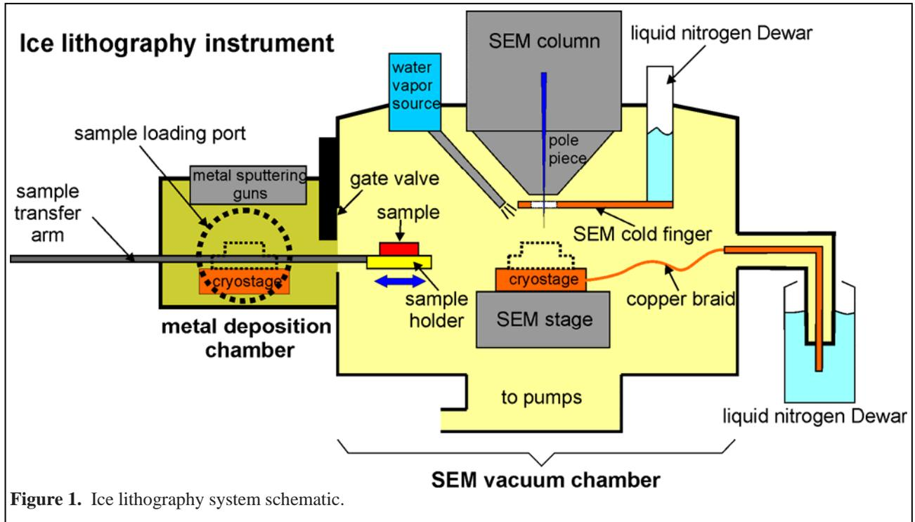
Figure 1. Ice lithography system schematic.
