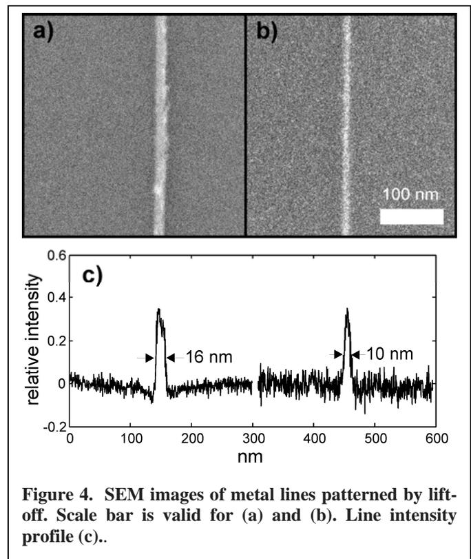
**Figure 4.** SEM images of metal lines patterned by lift-off. Scale bar is valid for (a) and (b). Line intensity profile (c).
