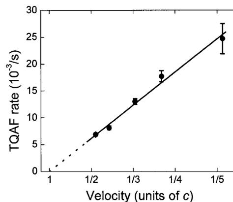
FIG. 4. TQAF event rate as a function of the inverse velocity of the positrons impinging on the plain carbon foil. The line is a fit of the  $c/v$  dependence to the data. Statistical error bars are shown. Towards larger velocities ( $v/c \rightarrow 1$ ), where the approximation breaks down, the line is dashed.
