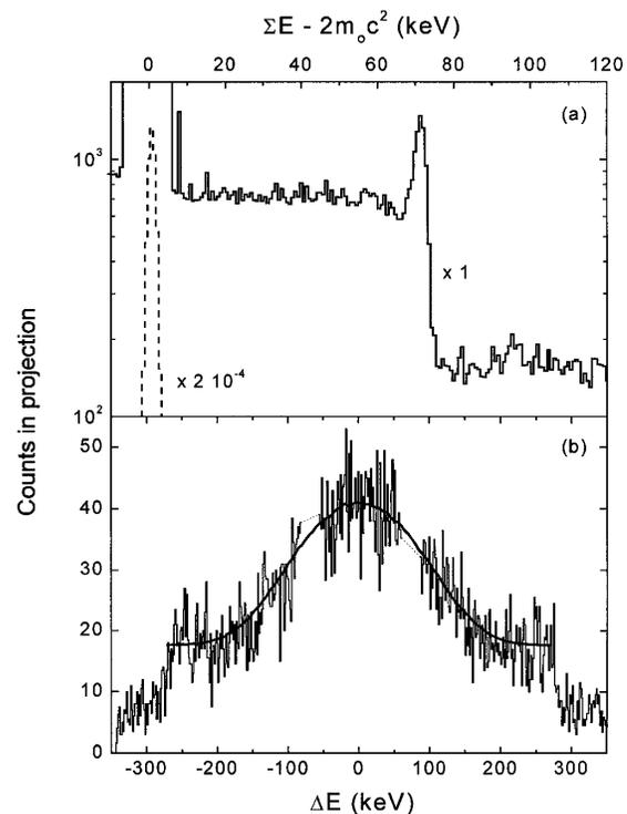
FIG. 2. Projection results in the difference energy direction (a) and the sum energy direction (b) from the data in Fig. 1. Part (a) consists of an integration across the full  $\Delta E$  width after the ridge elimination. The dashed line is the thermal peak part reduced by a factor of  $2 \times 10^{-4}$ . In part (b) the integration was performed across 10 keV centered at 71.6 keV  $\Sigma E$ . The smooth line is based on Eq. (2) folded with the angular resolution of the system.
