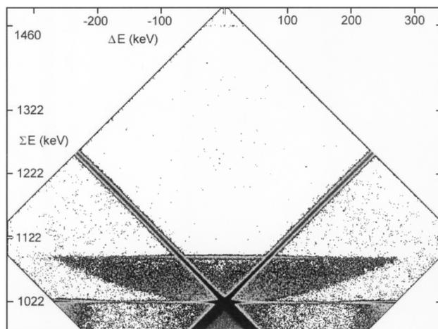
FIG. 1. 2D histogram of TQAF data from Au sputtered onto a C foil spanned by  $\Delta E$  ( $x$  axis) and  $\Sigma E$ . Counts are color coded from  $\leq 1$  (white) to  $10^2$  and larger (black) per bin on a  $\log_{10}$  scale. To enhance features with few counts all bins with more than 100 counts were set to 100.
