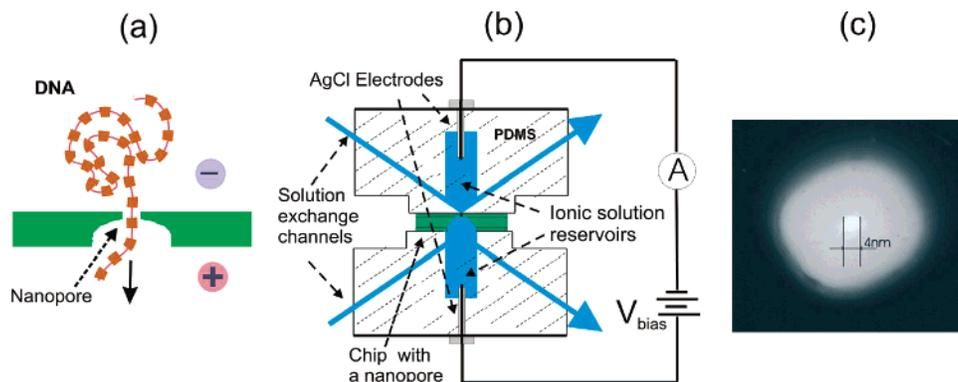
**Figure 1.** (a) Schematic illustration of DNA molecule translocating through a solid-state nanopore. (b) Experimental setup for single molecule measurements with a nanopore detector. (c) TEM of a silicon nitride nanopore, in this case 4 nm in diameter in a  $\sim 5\text{--}10$  nm thick local membrane.
