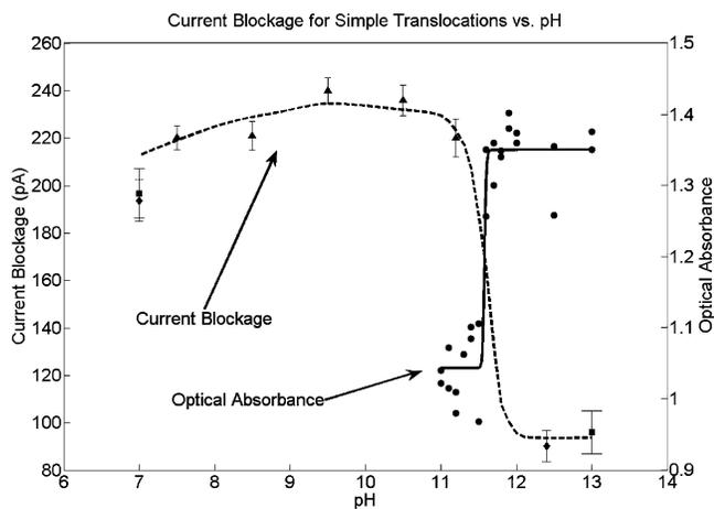
**Figure 3.** Plot of mean current blockage (for simple, unfolded, single level) events and DNA optical absorbance as a function of pH showing transition from ds to ss-DNA at pH  $\sim 11.5$ . The square markers represent the data from Figure 2, whereas the triangle and diamond markers represent experiments in two other pores including that in Figure 1c. The dashed line is a guide to the eye and not a fit.
