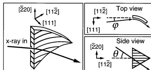
Fig. 1. Relative orientations of an incident x-ray beam and a bent Si(111) waveguide. Parallel curves indicate  $(\bar{2}20)$  lattice planes. The synchrotron radiation  $\mathbf{E}$  field is horizontal, normal to the waveguide surface, and parallel to the  $(\bar{2}20)$  lattice planes.
