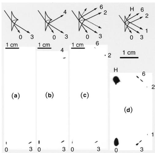
Fig. 2. Schematic beam-path and film exposures taken at (a)  $\theta - \theta_B = 1.745$  mrad, (b)  $\theta - \theta_B = -0.122$  mrad, and (c)  $\theta - \theta_B = 0$  mrad for 17.5-keV x rays on a  $R = 15$  cm Si(111) waveguide with grazing angle  $\varphi = 0.5$  mrad. (d)  $\theta = \theta_B$ ,  $R = 10$  cm,  $\varphi = 0.75$  mrad.
