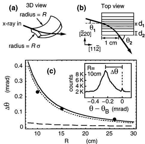
Fig. 3. (a) and (b) X-ray path on a bent Si plate with a saddlelike surface and a relaxed lattice. (c) Inset,  $\theta$  scan showing the dynamic diffraction peak at  $\theta = \theta_B$  and the edge diffraction peak at  $\theta - \theta_B = -0.231$  mrad for 17.5-keV WG x-rays on a  $R = 10$  cm Si(111) waveguide. The graph shows the angular separation of the two peaks,  $\Delta\theta = |\theta - \theta_B|$ , as a function of  $R$ .
