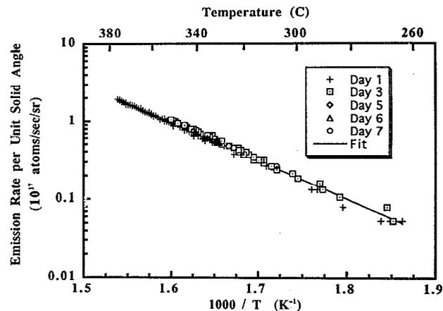
FIG. 2. Sodium emission rate per unit solid angle as a function of temperature. The different sets of data points correspond to different series of measurements and show the stability of the source. Note the exponential dependence on inverse temperature.
